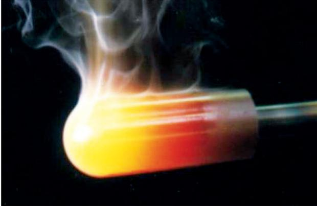
Refractory materials like molybdenum are choice materials for their mechanical, electrical, process, corrosion, and cost conditions required for the glass melting process.
